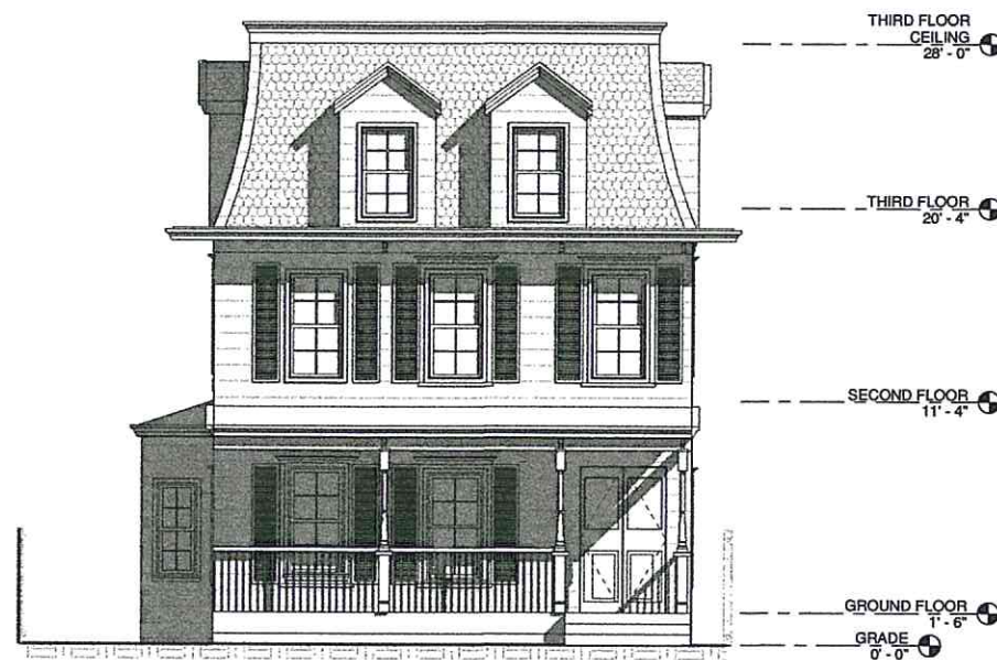
② EXISTING NORTH ELEVATION 1/4" = 1'-0"
