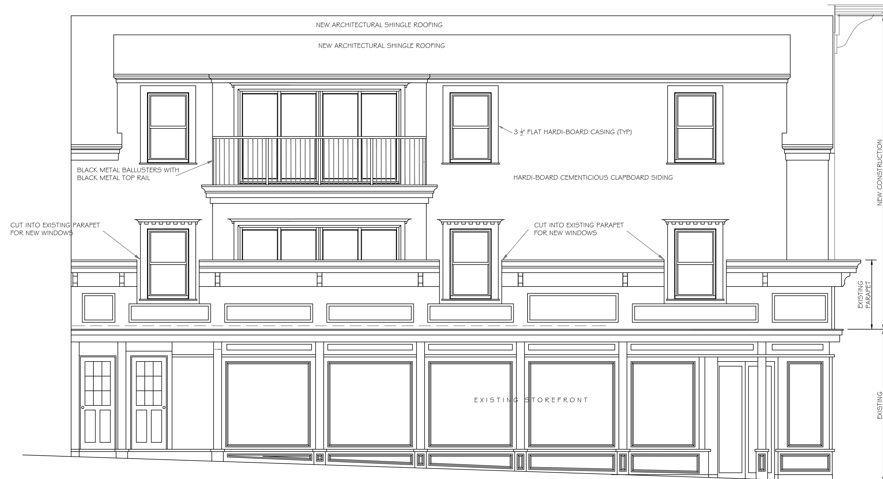
NORTH ELEVATION 1 AI SCALE : 1/4" = 1'-0"
