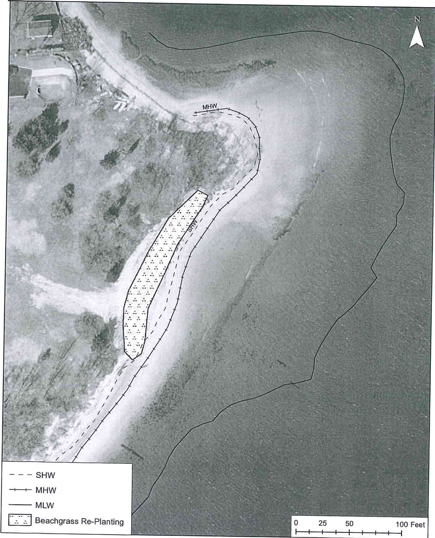
Figure 5. The area expected to be replanted with American beachgrass once dune repair work has been completed. The revegetation area encompasses approximately 4000ft 2 and will require 3,000-4,000 beachgrass culms.
