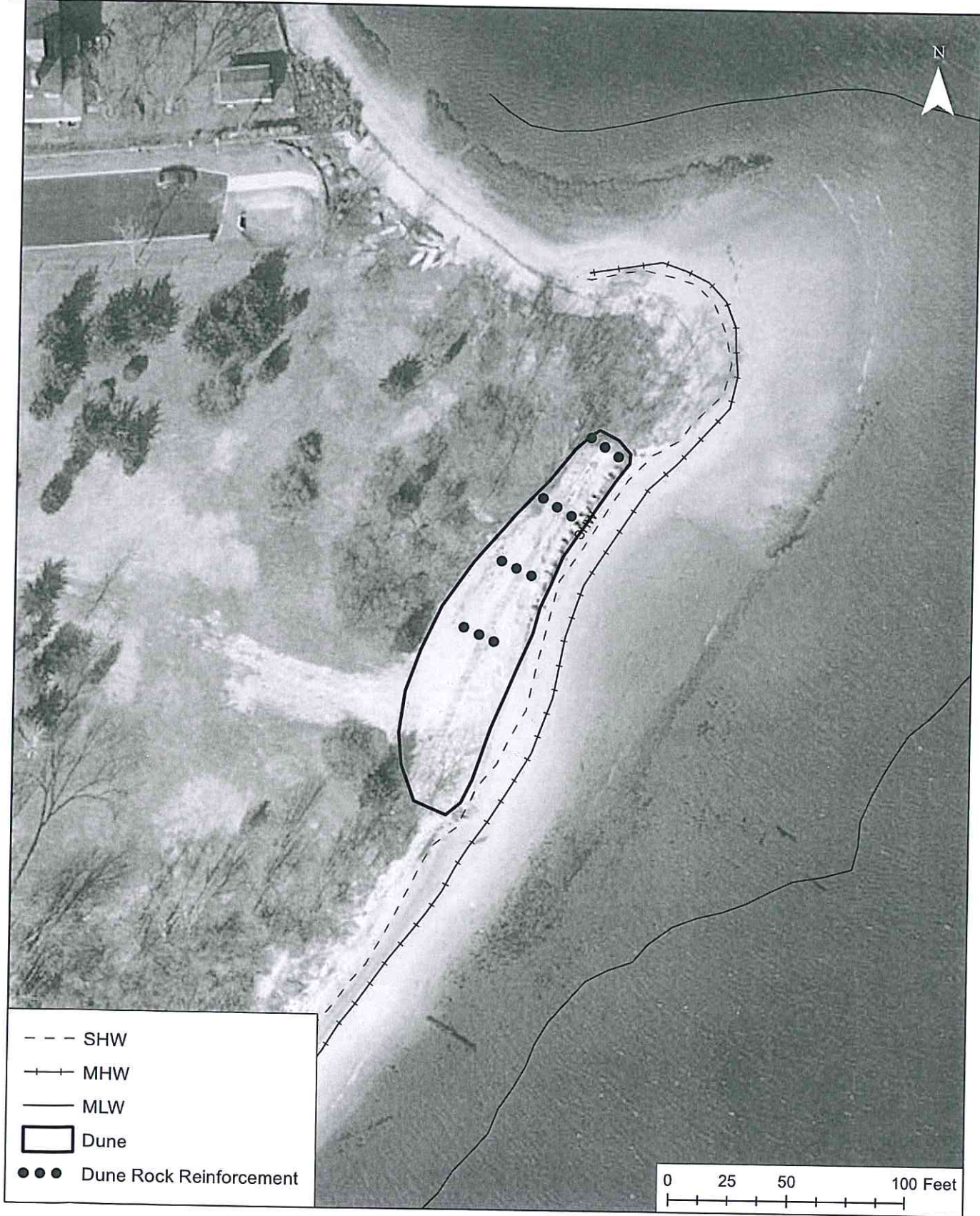
Figure 3. Location of the four, 15-foot boulder sections that will be placed perpendicular to, and extending upshore from, the existing boulder toe to reduce the chance of washout along the dune face if wave get behind the toe during a storm event.
